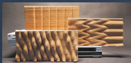
Textured samples made from 3D-printed raw earth taken before the water erosion test.
